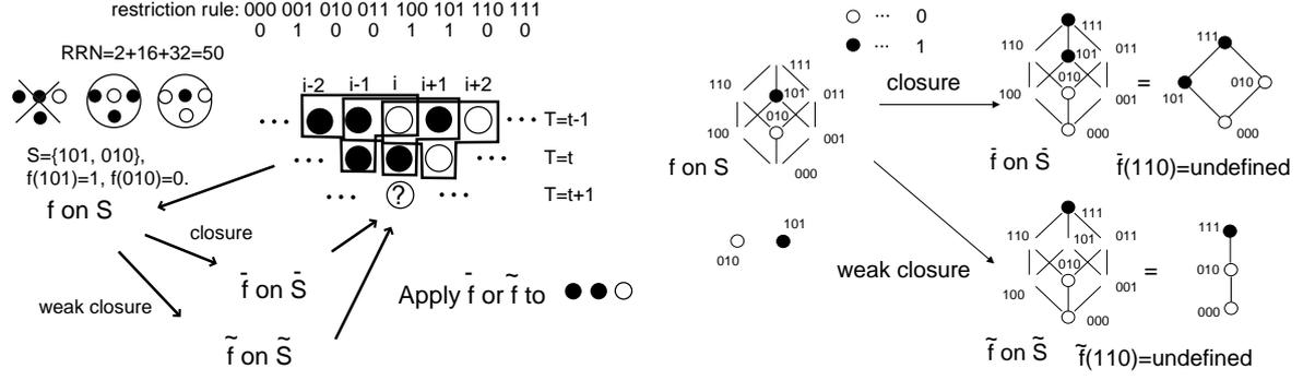
**FIGURE 2.** The time developmental procedures at site  $i$  and time  $t$  in both CD- and WCD-RLCA with  $RRN=50$  are shown (Left). Coressponding  $f, \bar{f}$  and  $\tilde{f}$  are also shown(Right).
